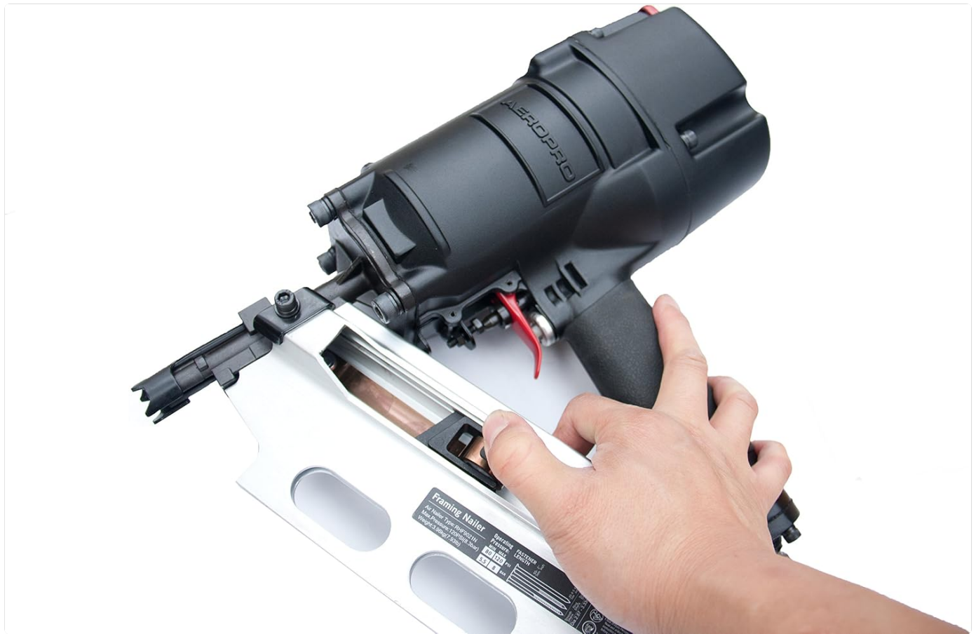
Figure 3.1: A hand demonstrating the process of loading nails into the nailer's magazine.
