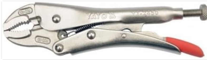
Figure 3.1: YATO YT-2450 Locking Pliers with adjustment screw visible. This image highlights the adjustment screw at the end of the handle, used to set the jaw opening and clamping pressure.
