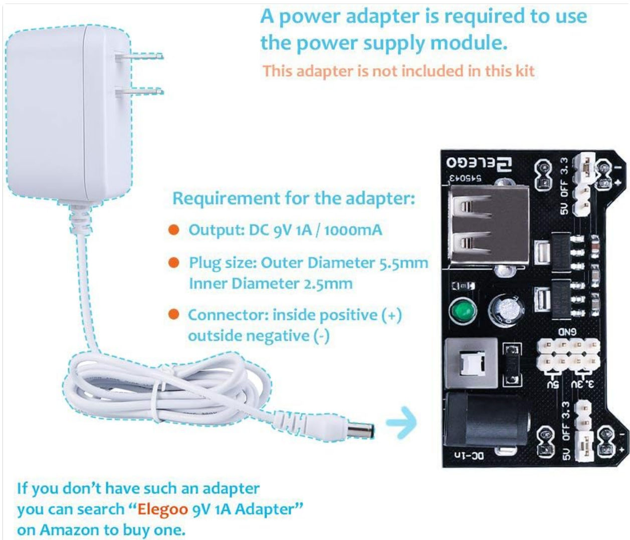
Image 3.2: Illustration of the required power adapter specifications for the Elegoo power supply module. It details the output, plug size, and polarity for proper connection.
