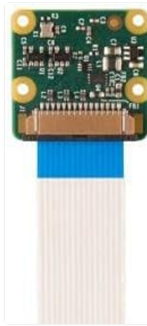
Figure 2: Rear view of the camera module, highlighting the ribbon cable connector.
