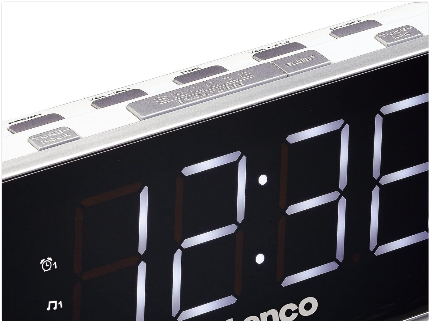
Figure 2: Close-up view of the top panel, showing the various control buttons such as TIME, ALARM 1/2, SNOOZE/BRIGHTNESS, VOL+/-, TUNE+/-, PRE/M+, and ON/OFF. The rear panel typically houses the power input and FM antenna.
