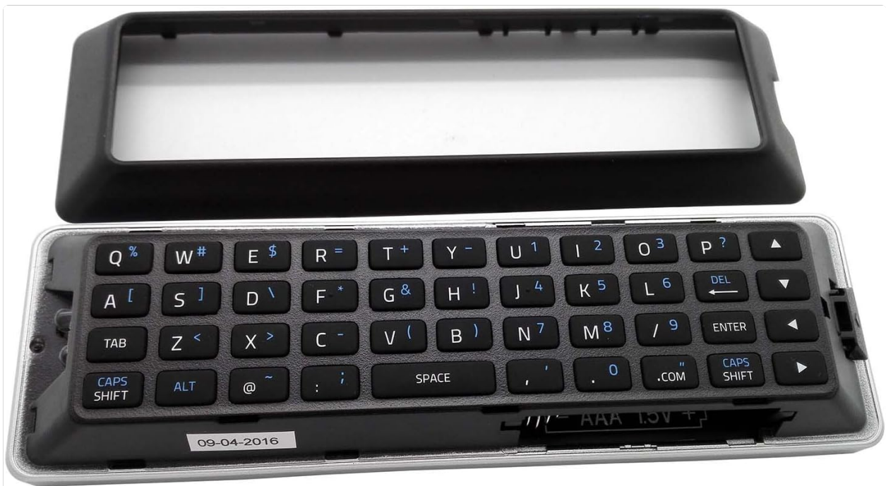
Image: The VIZIO XRT500 remote with its battery compartment open, showing the placement for two AAA batteries.
