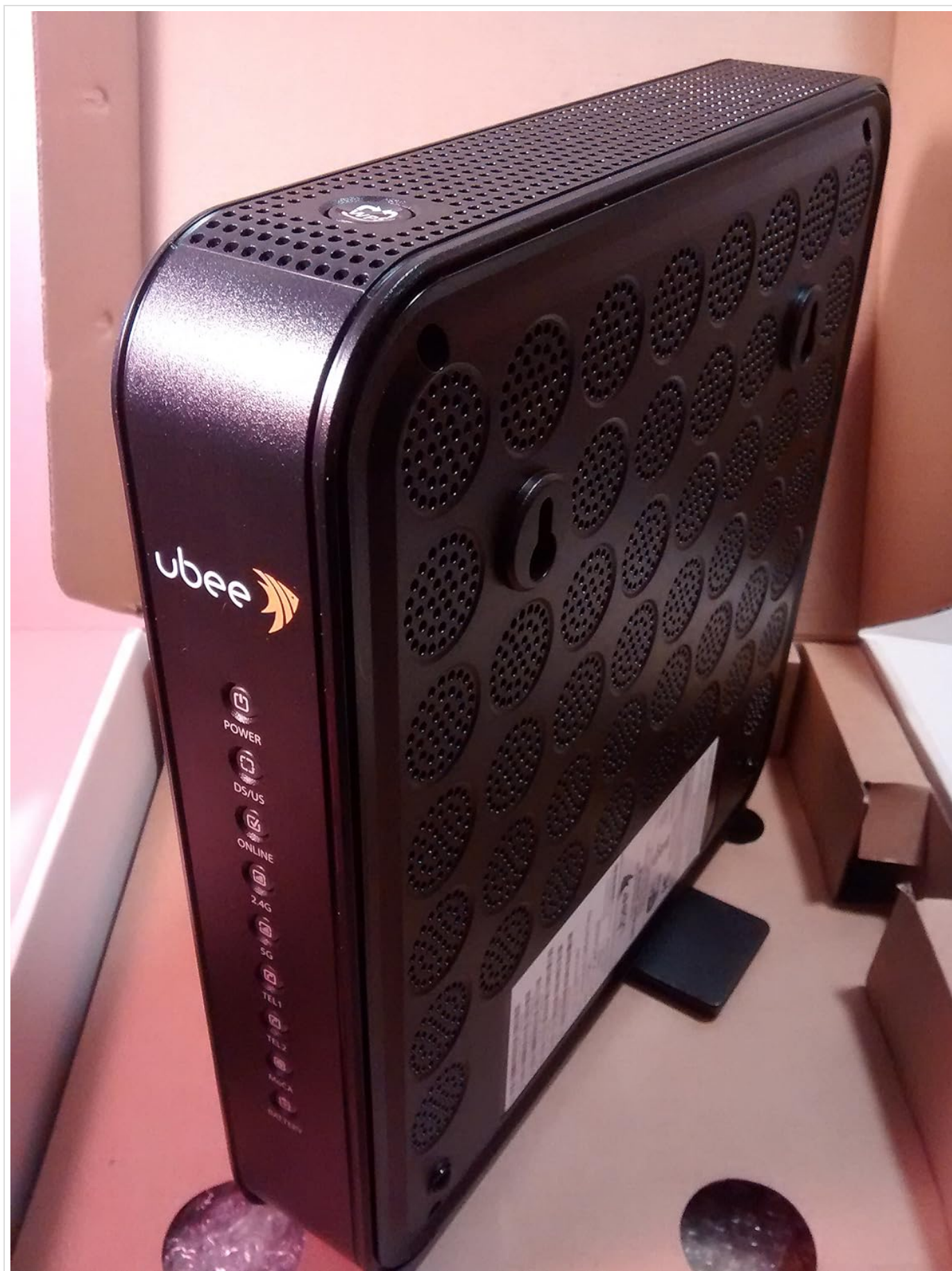
Figure 1: Side view of the Ubee DVW32CB showing the LED indicators for Power, DS/US, Online, 2.4G, 5G, TEL1, TEL2, and Battery.
