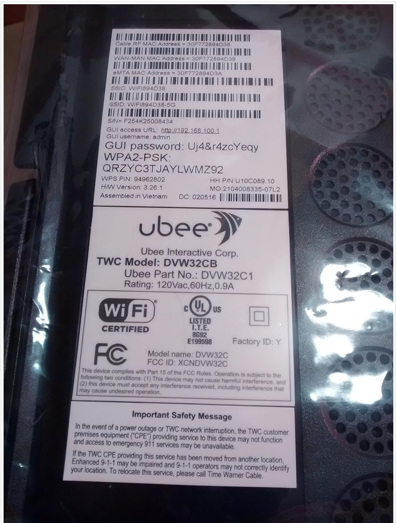
Figure 3: Product label displaying network information such as SSID, WPA2-PSK, MAC addresses, and serial number (S/N: F254K25008434). The manufacturing date code (DC: 020516) is also visible.
