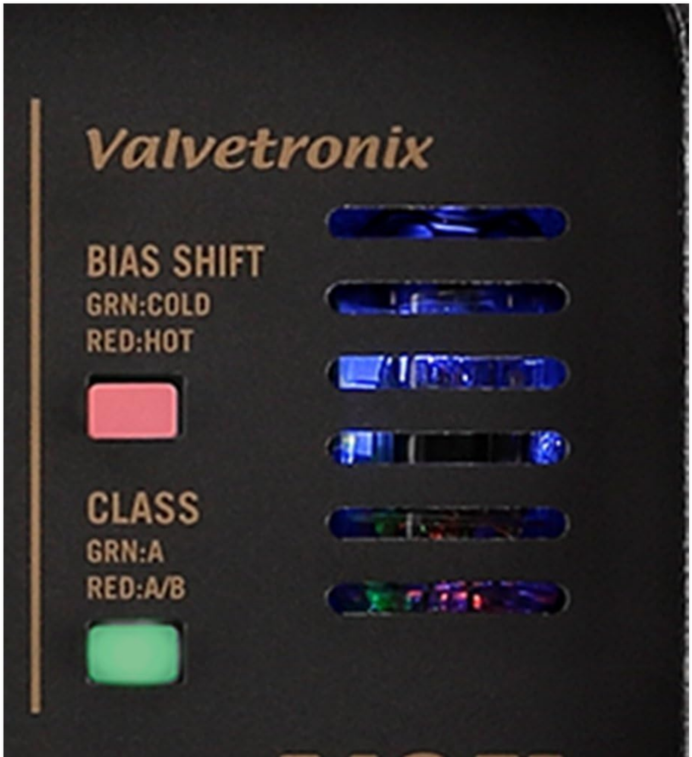
Figure 4: Close-up view of the Valvetronix section, showing BIAS SHIFT (GRN:COLD, RED:HOT) and CLASS (GRN:A, RED:A/B) indicators, which reflect the vacuum tube's operational state.
