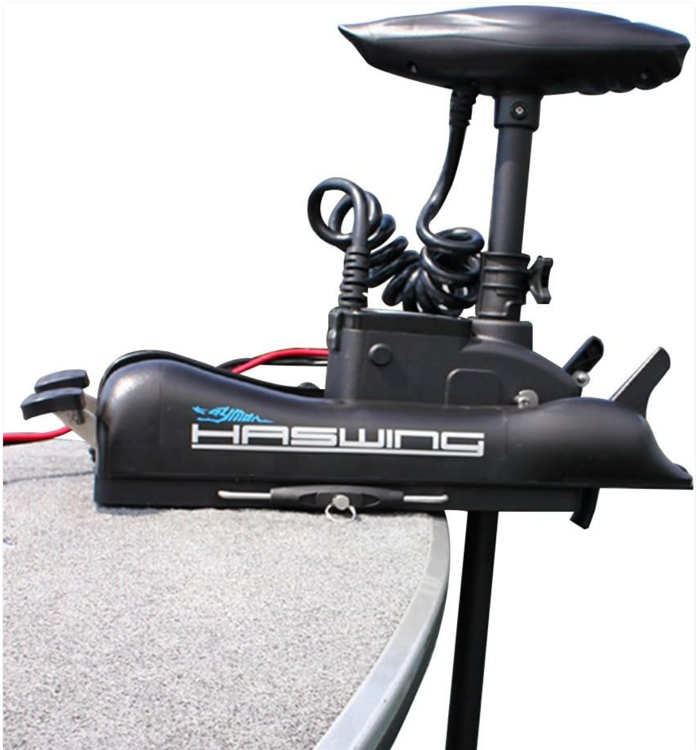
Image: A Haswing trolling motor securely mounted on the quick release bracket, attached to the bow of a boat.
