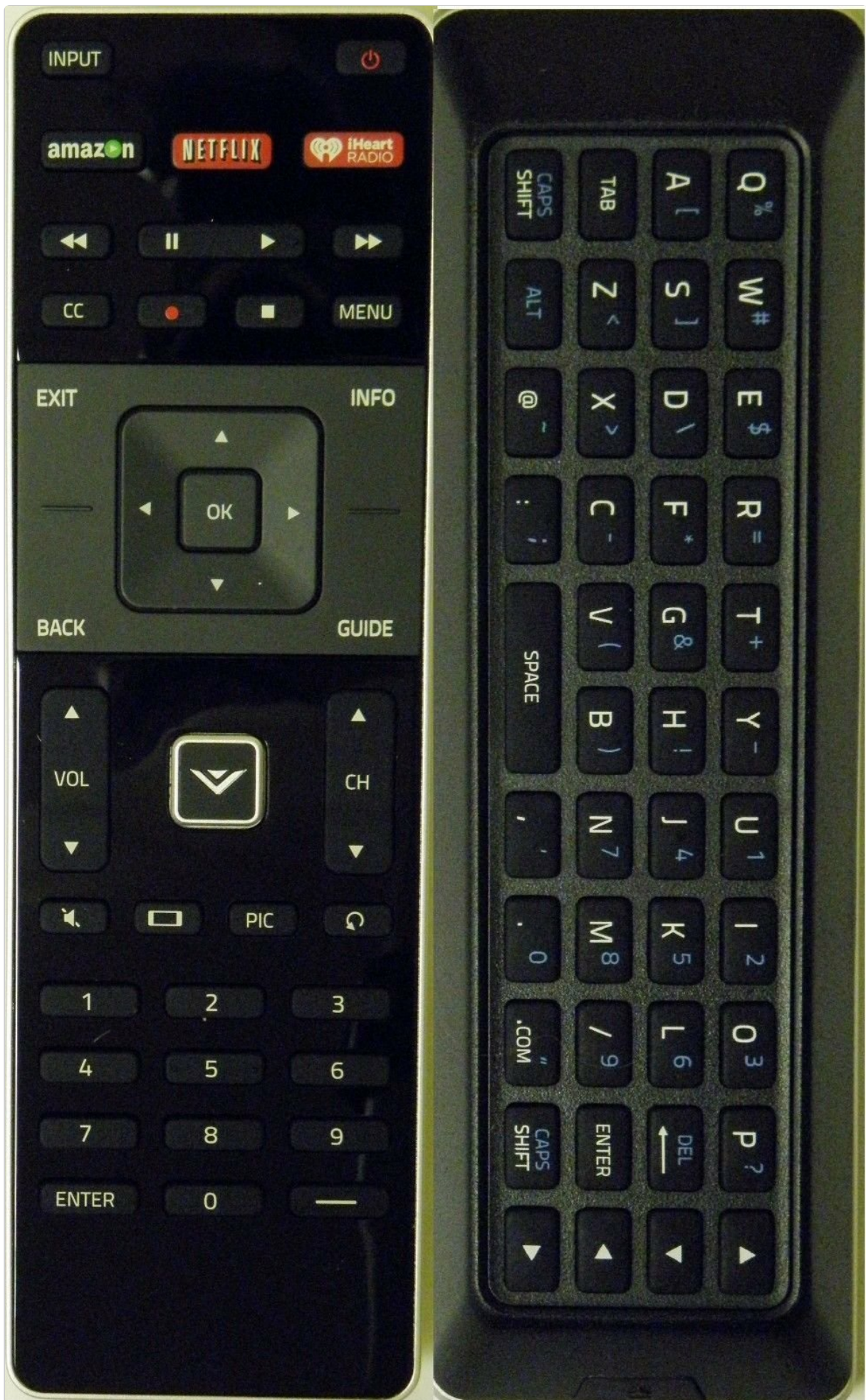
Image: The VIZIO XRT500 Remote Control, displaying its primary control side on the left and its full QWERTY keyboard on the right. The primary side includes power, input, channel, volume, navigation, and dedicated app buttons. The keyboard side features alphanumeric keys, shift, caps, tab, and directional arrows.
