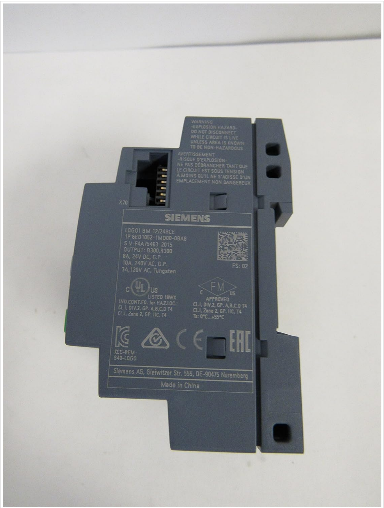
Figure 3.3: Side view of the Siemens Logo 8 PLC, showing product labels, certifications, and the Ethernet port (X70).
