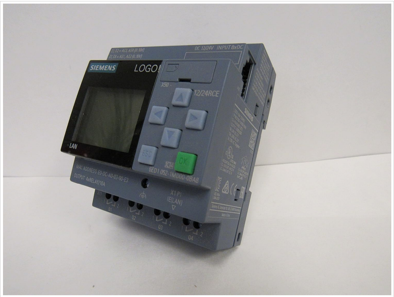
Figure 3.1: Angled view of the Siemens Logo 8 PLC, showing the display, control buttons, and various connection terminals.
