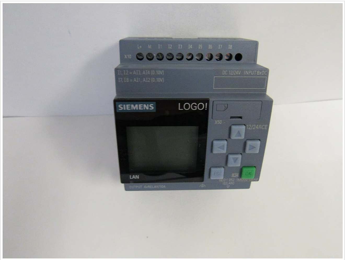
Figure 3.2: Front view of the Siemens Logo 8 PLC, highlighting the integrated display and navigation buttons for direct device interaction.
