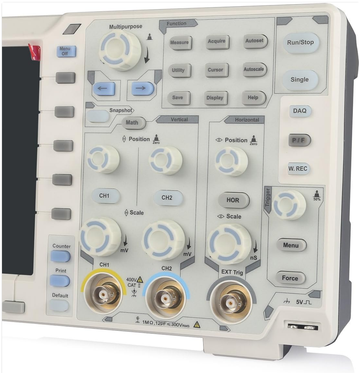
Figure 5: Detailed view of the front panel, showing CH1 and CH2 BNC input connectors and associated controls.
