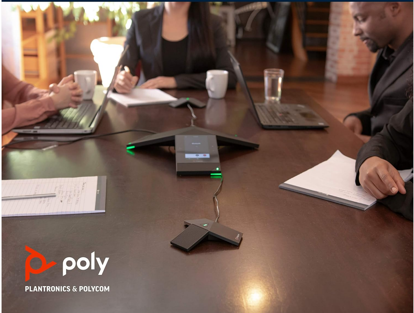
Image 3.1: A Polycom Trio conference phone centrally placed on a meeting table, with two expansion microphones connected and positioned to extend audio coverage for participants.
