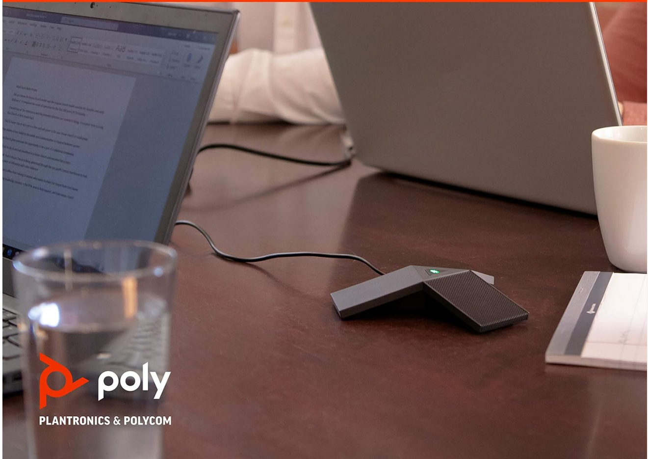
Image 3.2: A single Polycom expansion microphone positioned on a conference table, demonstrating its ability to capture audio from participants up to 20 feet away.
