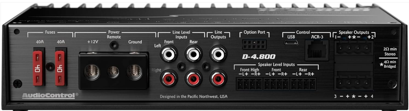
Figure 2: Rear panel of the AudioControl D-4.800 amplifier, showing power, ground, remote, line-level inputs, speaker-level inputs, line outputs, and speaker outputs.
