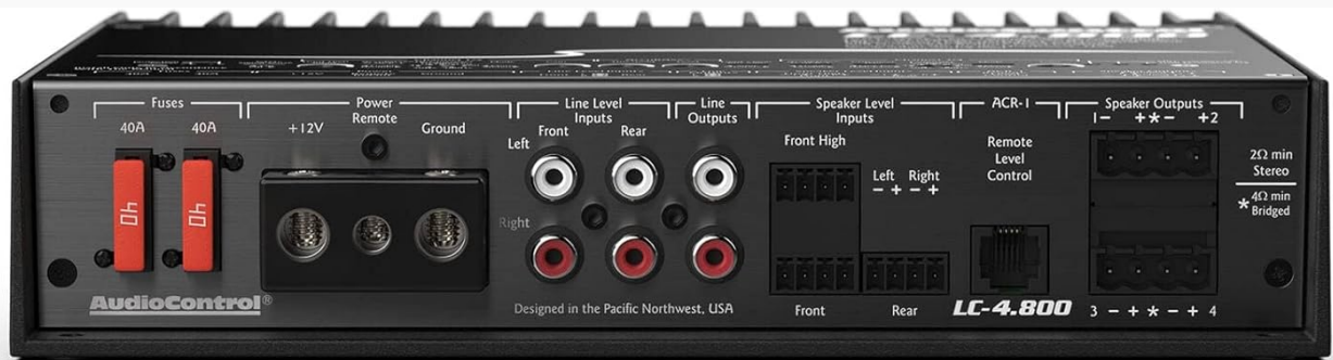
Figure 3.4: Detailed rear panel view of the LC-4.800 amplifier, showing all connection ports including fuses, power/remote/ground terminals, line-level inputs, line outputs, speaker-level inputs, remote level control port, and speaker outputs.
