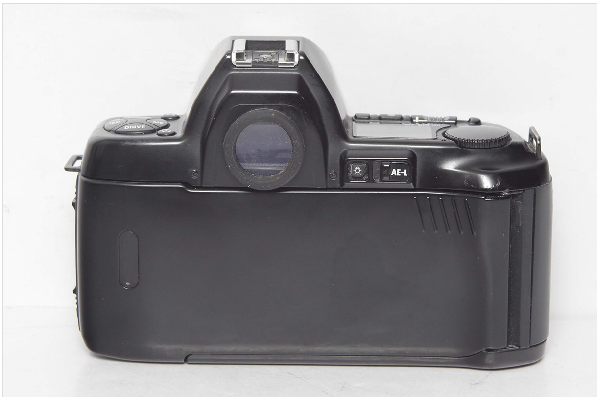
Figure 3: Rear view of the Nikon AF N8008 camera. This image displays the camera's viewfinder, the AE-L (Auto Exposure Lock) button, and the general layout of the back panel.
