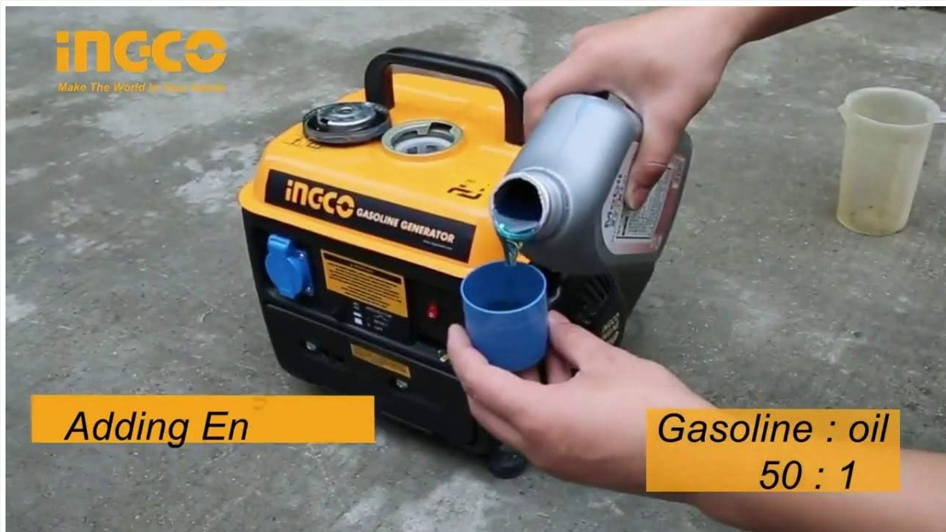
Figure 3.2: Illustration of adding fuel to the generator. This image shows the process of pouring gasoline into the fuel tank. Note: The image text "Gasoline : oil 50 : 1" suggests a 2-stroke mixture, but the product specifications clearly state "4-stroke engine". Follow the 4-stroke engine instructions for separate fuel and oil.
