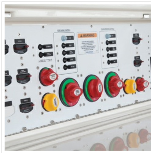
Figure 3: A marine electrical panel showing various switches and battery selectors, typical of systems managed by this conversion kit.
