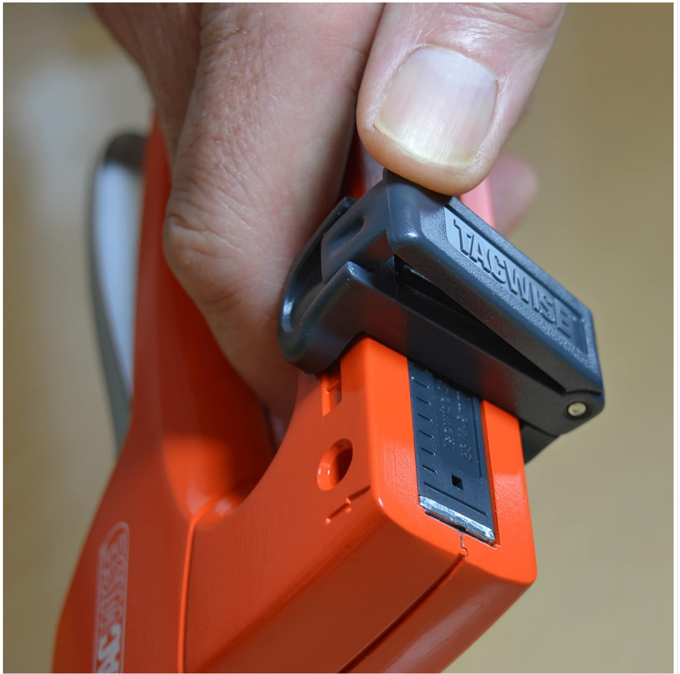
Figure 3: Operating the staple magazine release mechanism.
