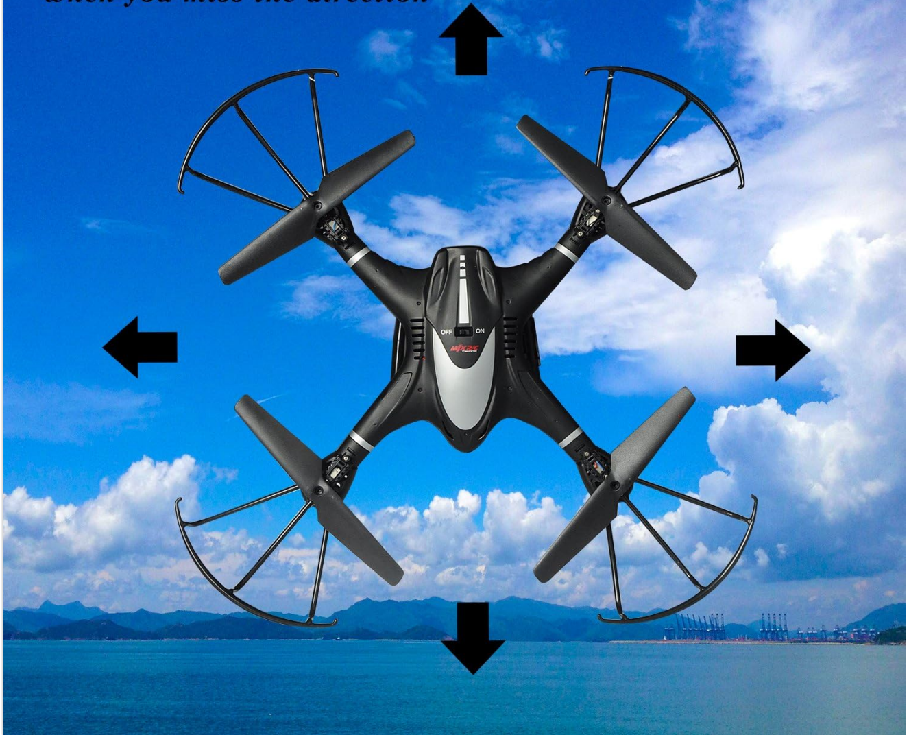
Figure 4.4.2: Depiction of Headless Mode, where the drone's orientation is relative to the pilot, simplifying control regardless of the drone's front direction.
