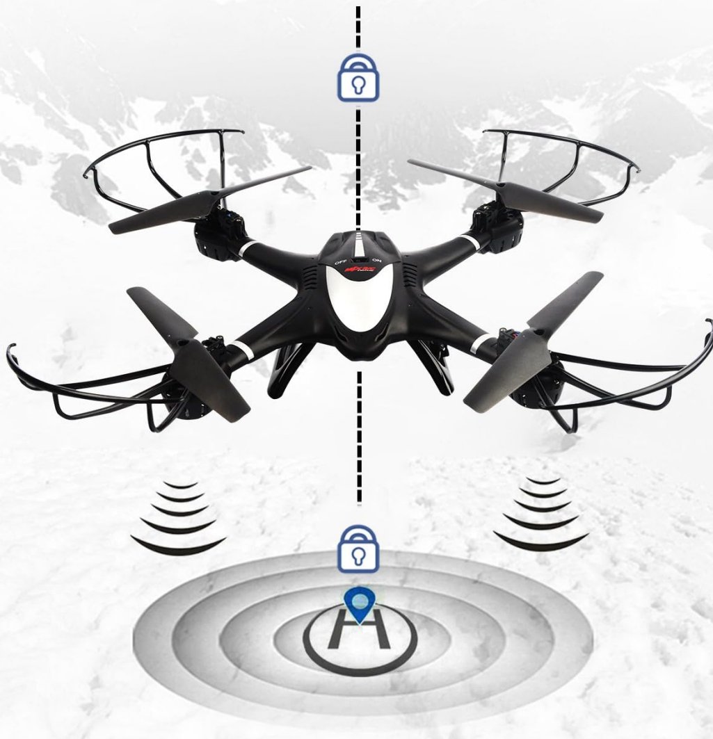
Figure 4.4.1: Visual representation of the Altitude Hold feature, where the drone automatically maintains a set height, indicated by a lock icon.
