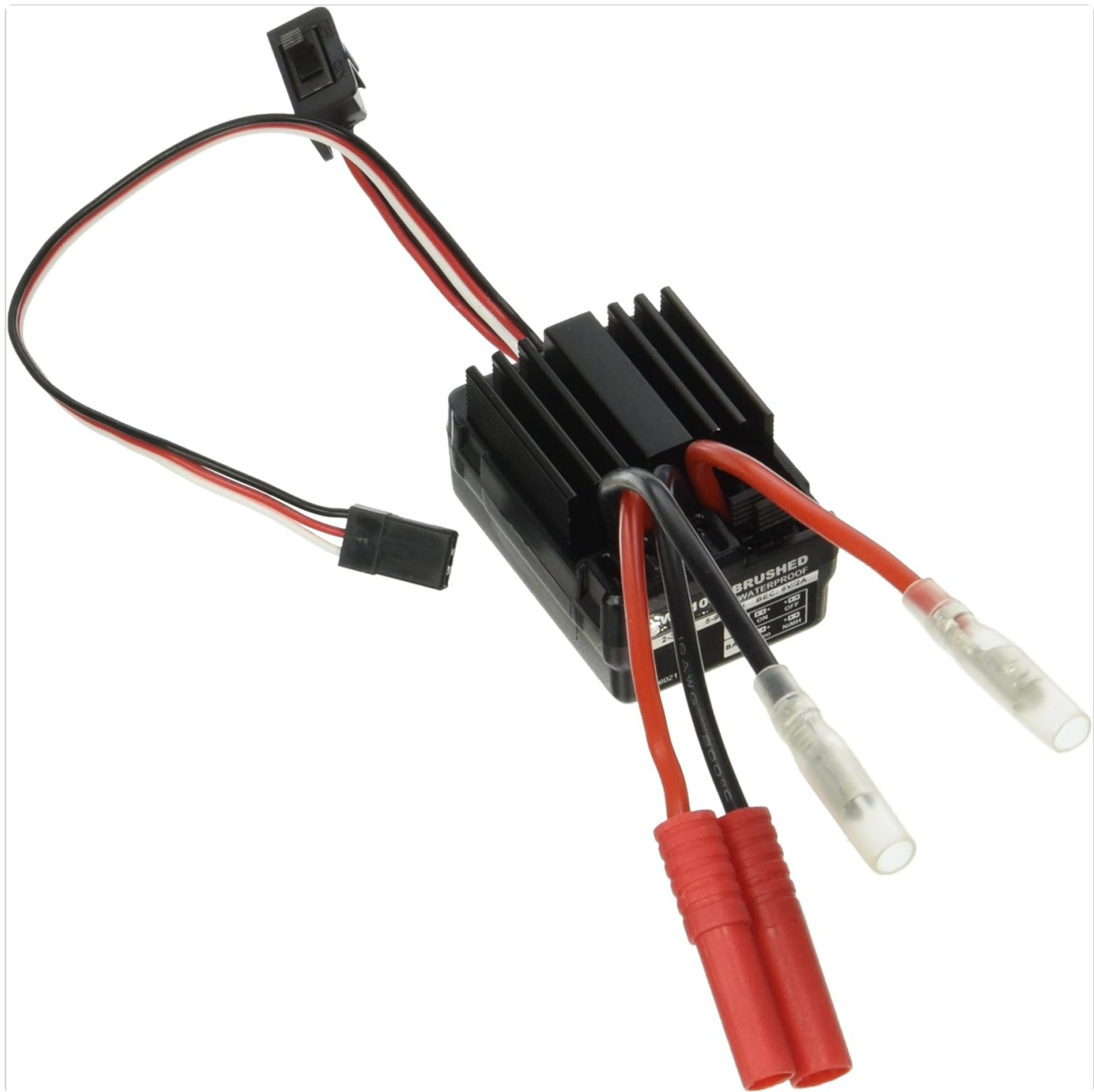
Figure 3.1: Redcat Racing Hobbywing 1/10 Brushed Waterproof Electronic Speed Control. This image displays the ESC unit with its black heat sink, red and black power wires connected to the battery and motor, and a smaller signal wire for the receiver. A power switch is also visible.
