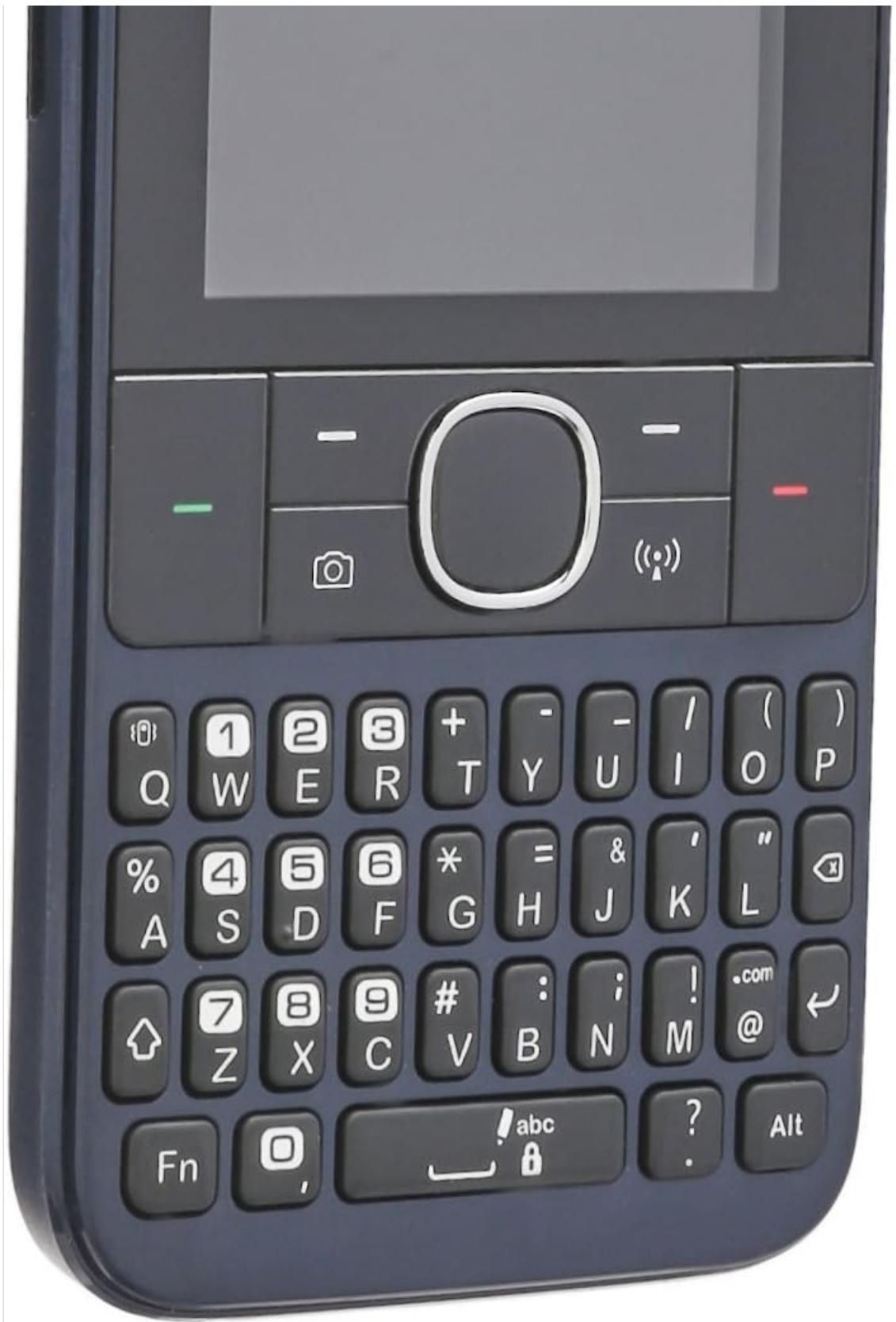
Figure 3.1: Front view of the Alcatel OT-3022G, showing the display, navigation keys, and QWERTY keyboard.
