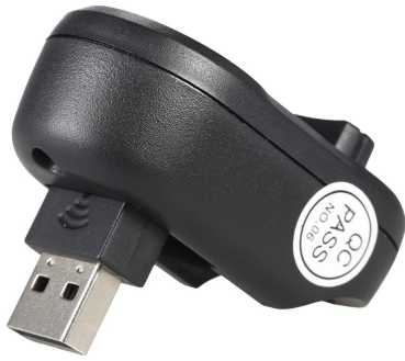
Figure 2: Side view of the GODOX XTR-16 receiver, highlighting its USB connector for integration with compatible flash units.
