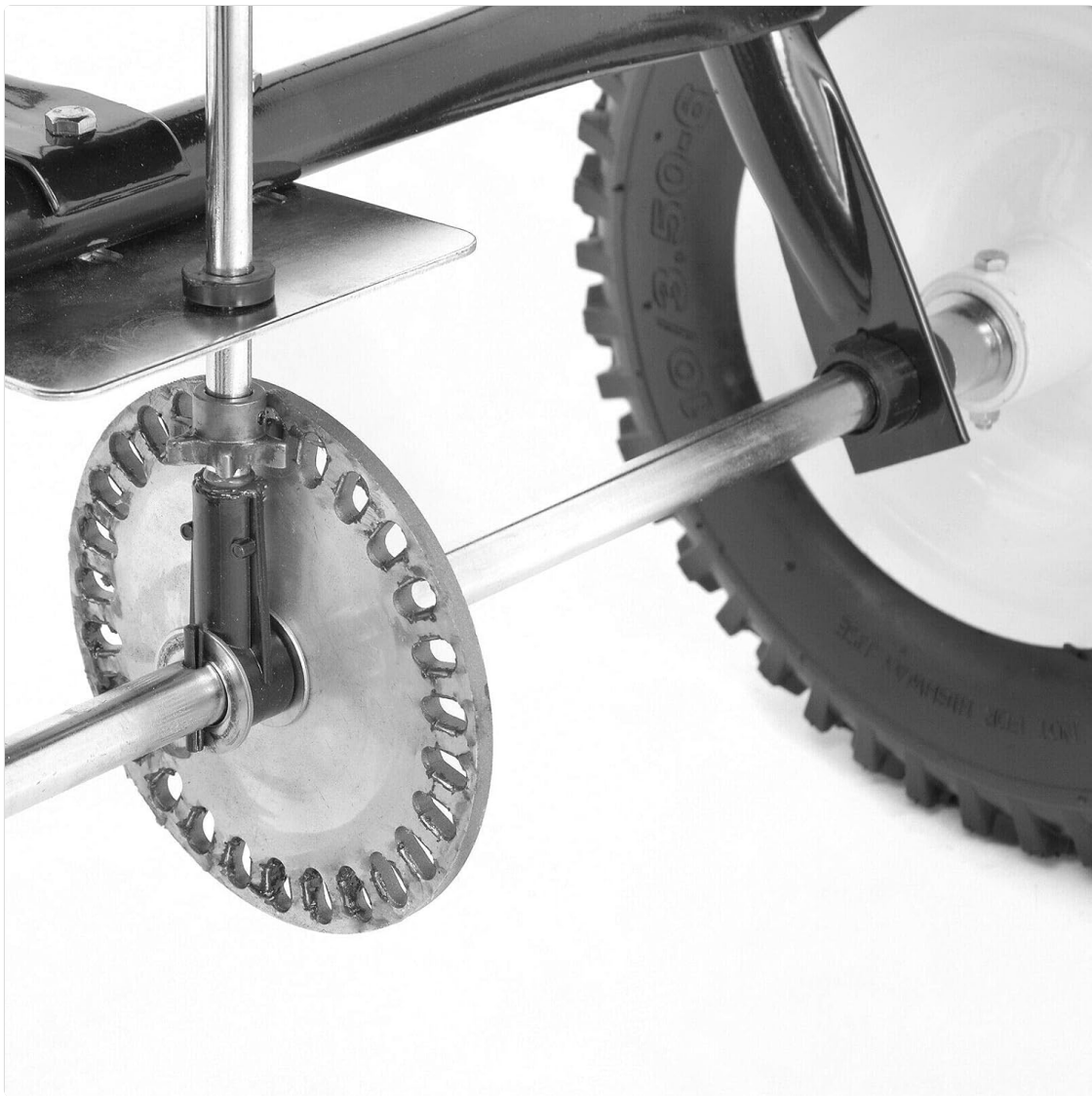
Figure 5: Detailed view of the gear and spreading plate mechanism. Verify that the agitator rod is properly seated.
