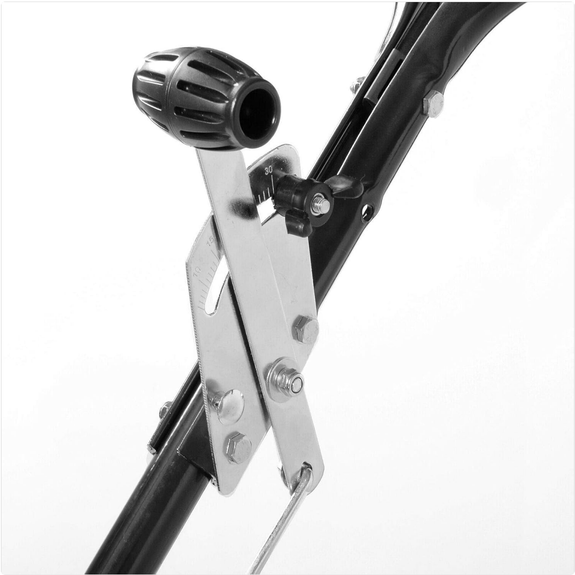
Figure 7: Detailed view of the control lever for adjusting the spreading rate. The lever includes an adjustable stop for precise flow limitation.
