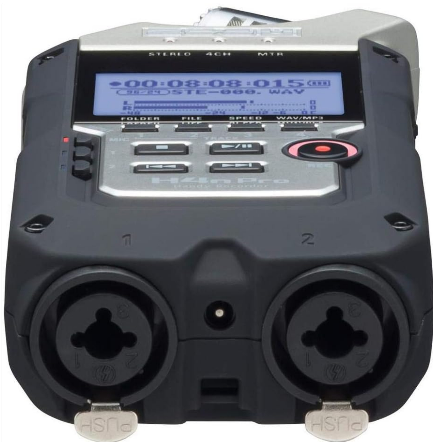
Figure 3: Bottom view of the Zoom H4n Pro, featuring the two XLR/TRS combo input connectors.
