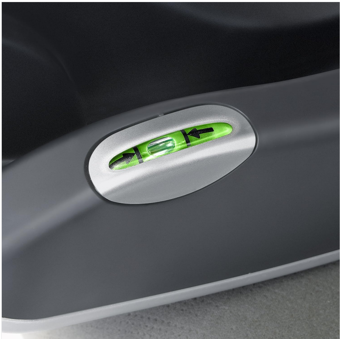
Figure 2: Adjusting the recline of the KeyFit 30 car seat base using the leveling foot.
