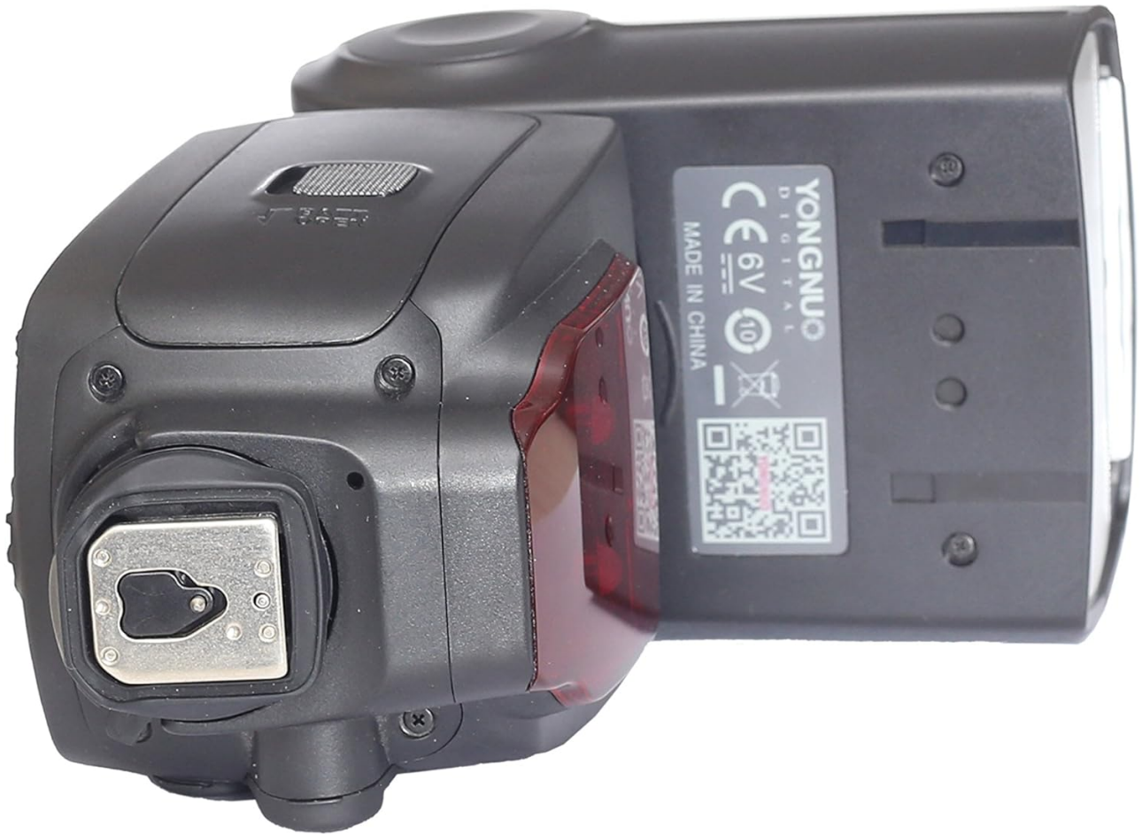
Figure 5.1: Bottom view of the YN660 Speedlite, illustrating the hot shoe and locking mechanism.
