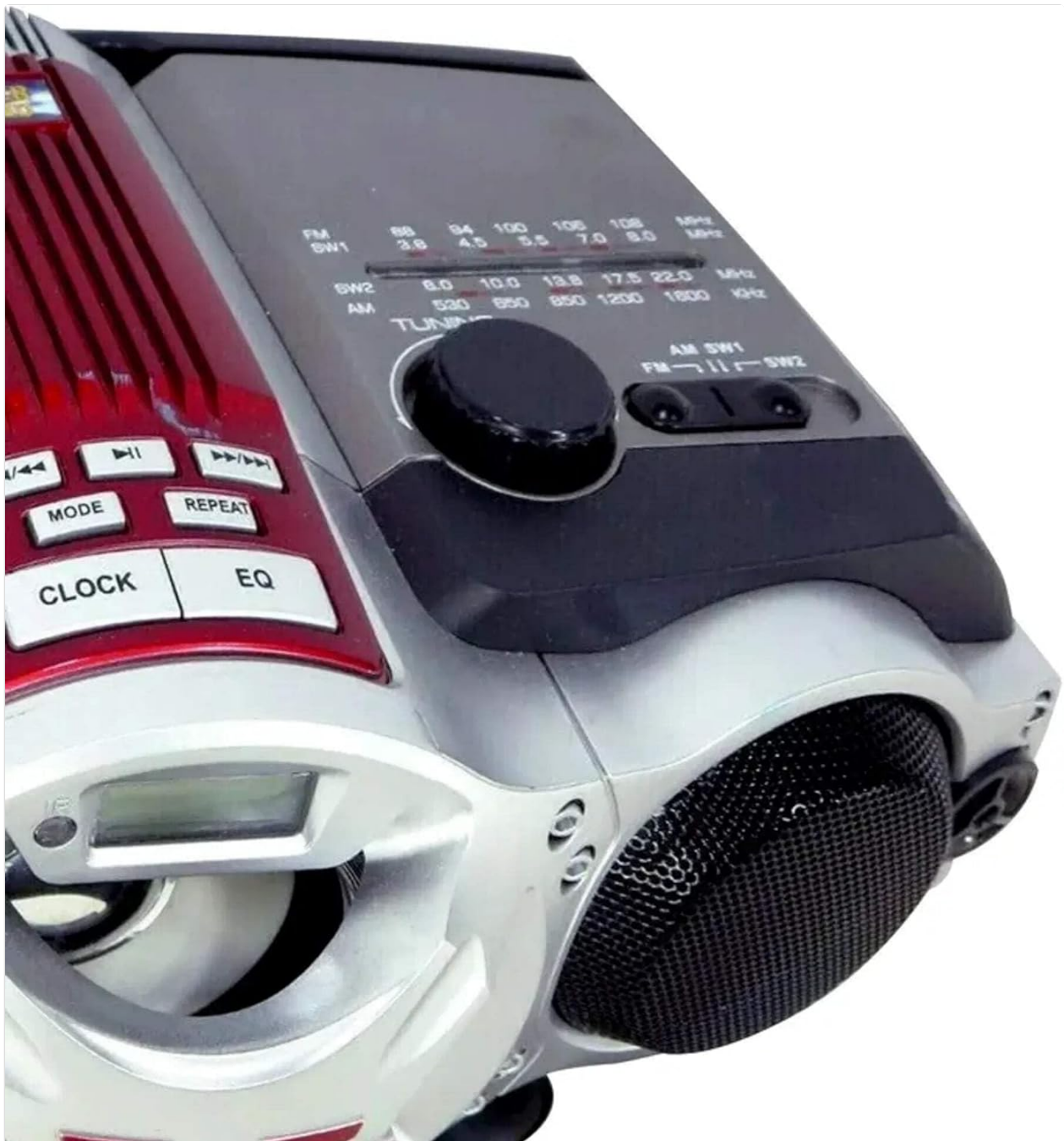
Figure 3: Right side controls, featuring the AM/FM/SW1/SW2 band selector, TUNING knob, and playback control buttons (Play/Pause, Skip, Mode, Clock, EQ).
