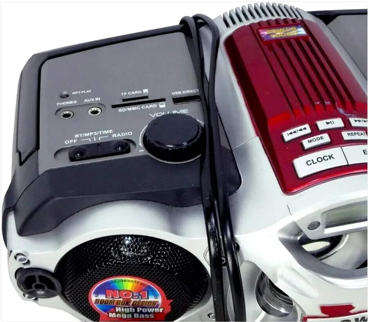
Figure 2: Left side controls, including USB input, SD/Micro SD card slot, AUX IN, PHONES jack, BT/MP3/RADIO mode switch, and Rotary Volume control.
