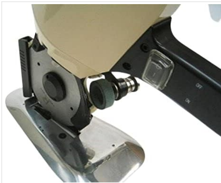
Figure 3: Close-up view of the Cutex RC-100 blade and sharpening mechanism. This detailed image highlights the 4-inch octagonal blade, the blade guard, and the integrated sharpening stone, which is crucial for maintaining cutting efficiency.
