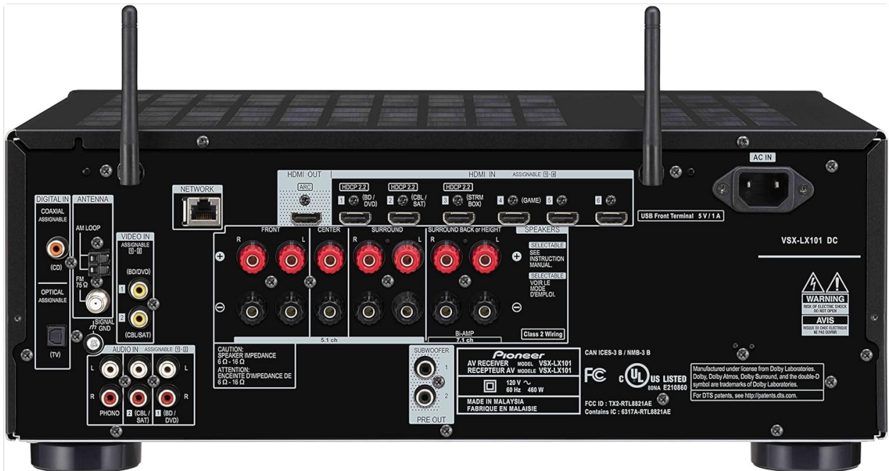
Figure 4.2: Rear Panel Connections. This image illustrates the rear panel of the Pioneer VSXLX101 receiver, detailing various input and output ports. It includes multiple HDMI inputs and one HDMI output with ARC support, digital audio inputs (optical and coaxial), analog audio inputs, video inputs, and speaker terminals for 7.2 channel configuration. Wi-Fi antennas and an Ethernet port for network connectivity are also visible, alongside the AC power inlet.
