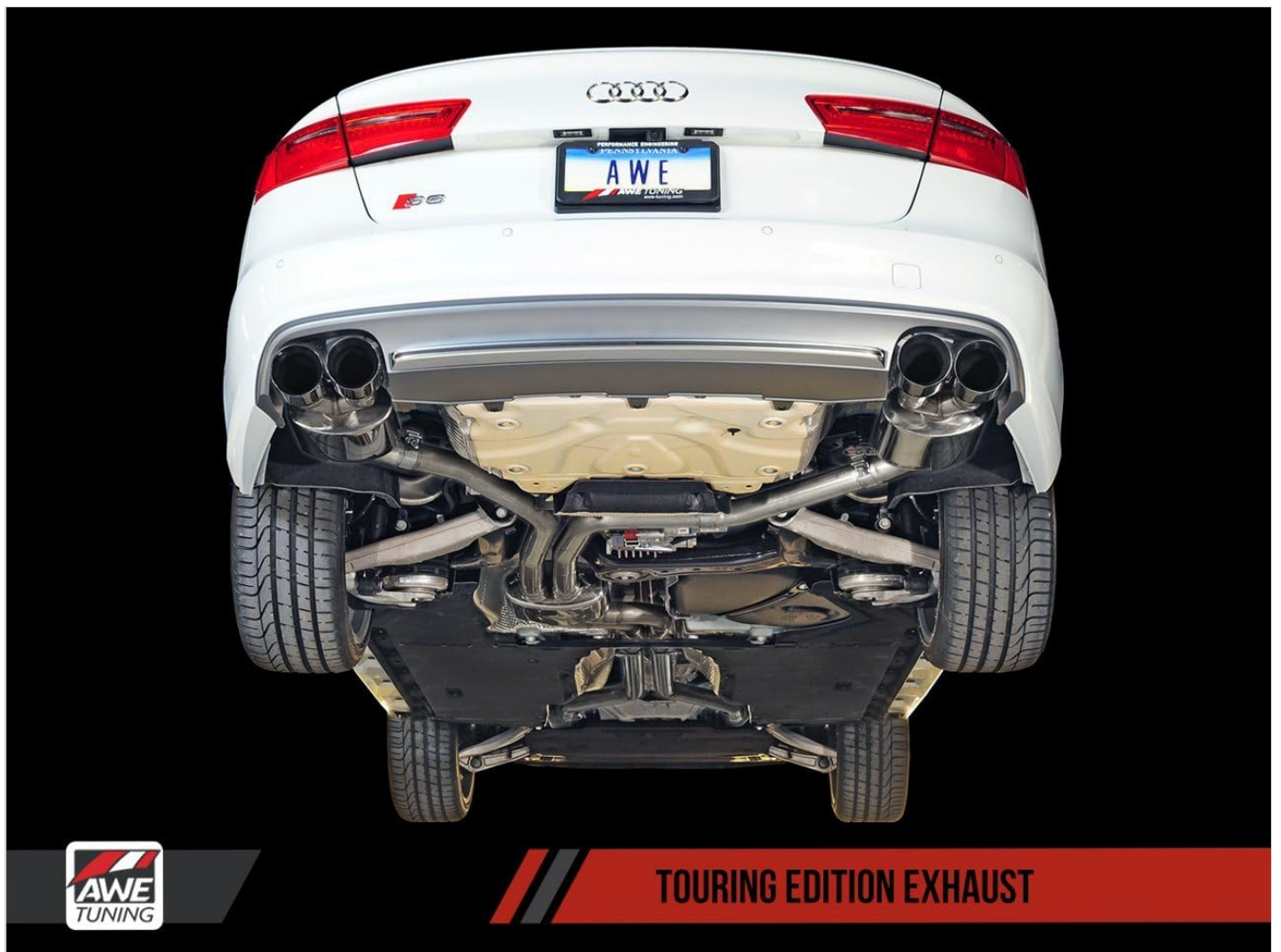
Figure 1: Undercarriage view of the AWE Tuning Touring Edition Exhaust System installed on an Audi S6, highlighting the 304 SS tubing and quad tip configuration.
