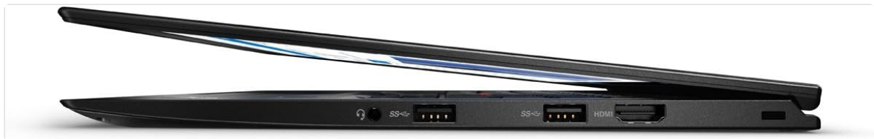
Figure 2: Left side of the laptop, illustrating the headphone/microphone combo jack, two USB 3.0 ports, and an HDMI port.
