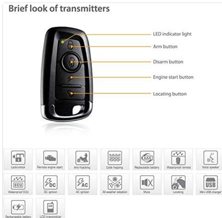
Figure 3: Standard Remote Control with button functions and feature icons.
