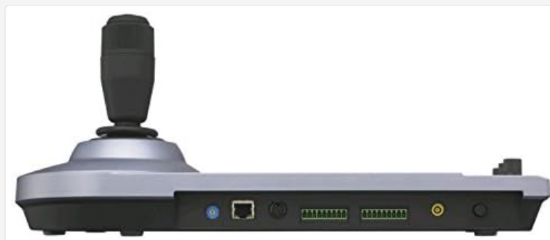
Figure 4.3: Rear panel of the RM-IP10, illustrating the connectivity options for network and external devices.
