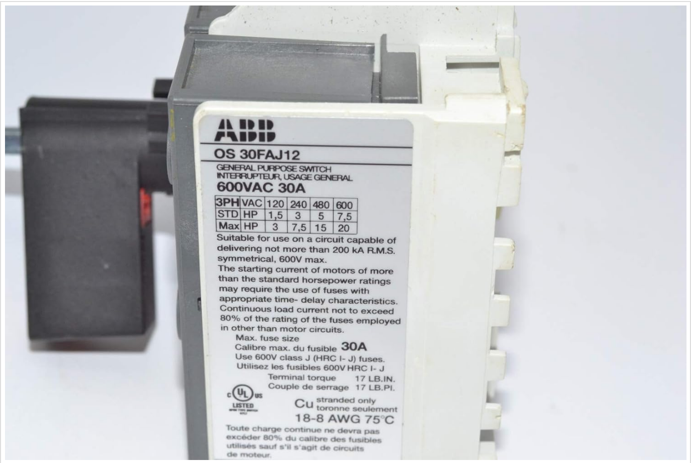
Figure 2: Side view of the disconnect switch, displaying the product label with model number OS30FAJ12, voltage ratings (600 VAC), horsepower ratings, and terminal torque specifications. This label provides critical information for correct wiring and application.
