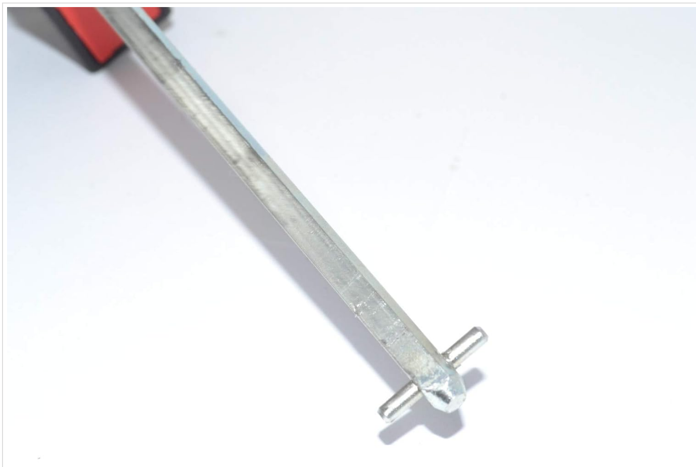
Figure 4: Close-up of the fuse puller tool, showing its design for safe and easy removal and insertion of fuses. This tool is essential for maintenance and fuse replacement.
