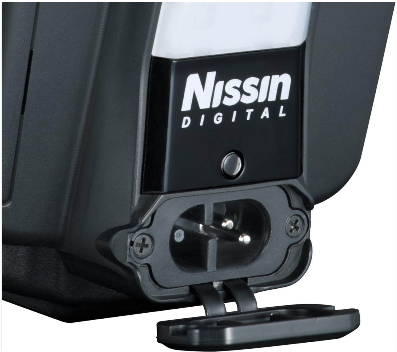
Image: The external power port on the side of the flashgun, used for connecting an optional power pack.
