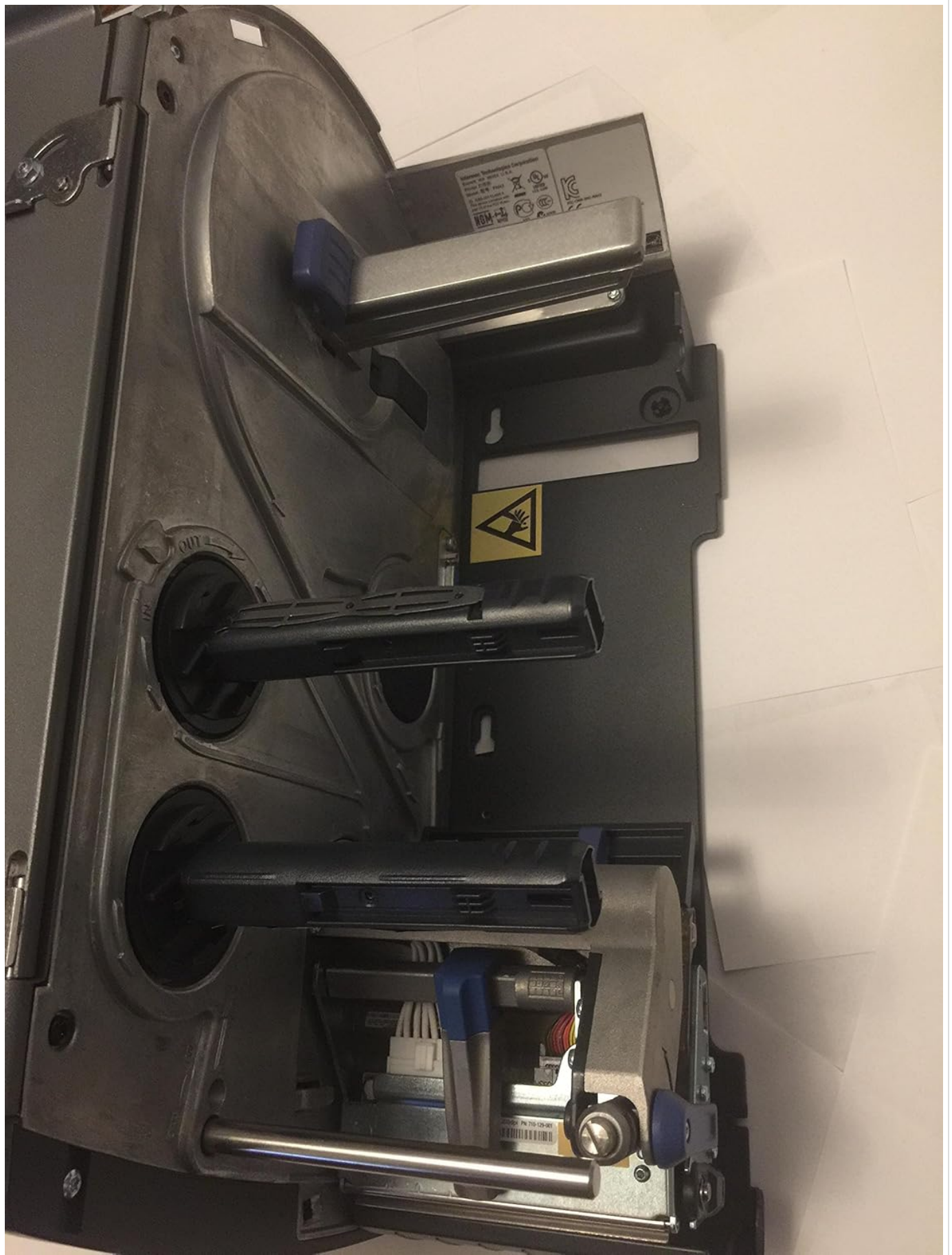
Figure 3: Internal view of the PM43 printer, highlighting the media and ribbon loading mechanisms.
