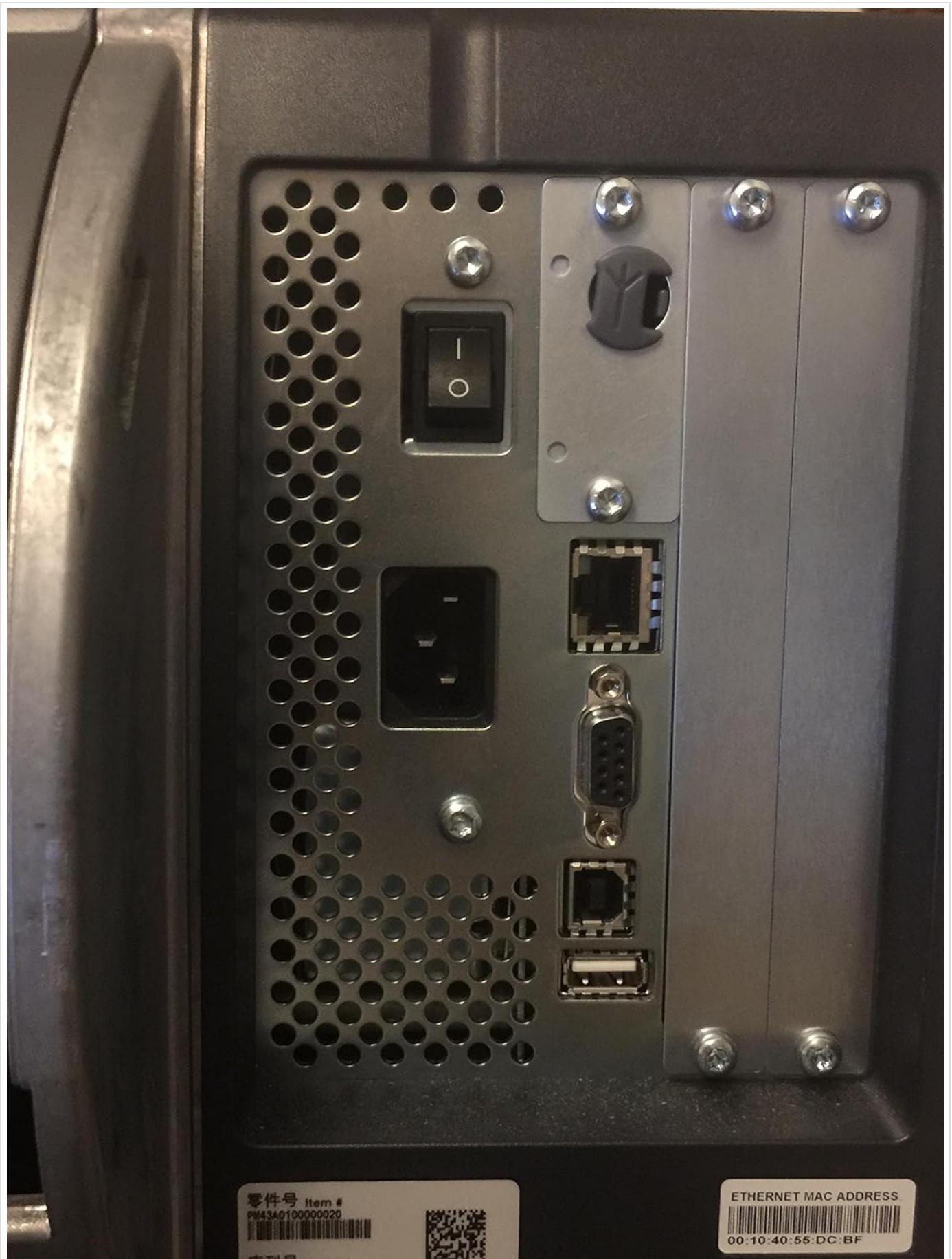
Figure 2: Rear panel of the PM43 printer, illustrating the power inlet, power switch, USB ports, and Ethernet port.
