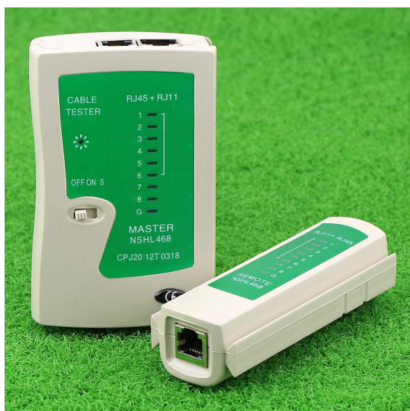
Figure 3.2: The NSHL-468 Network Cable Tester with its remote unit detached from the master unit. This separation allows for testing of cables that are already installed over long distances.
