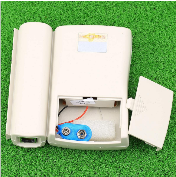
Figure 3.4: The open battery compartment of the NSHL-468 Network Cable Tester, showing the slot for a 9V battery. A 9V battery is required for operation.
