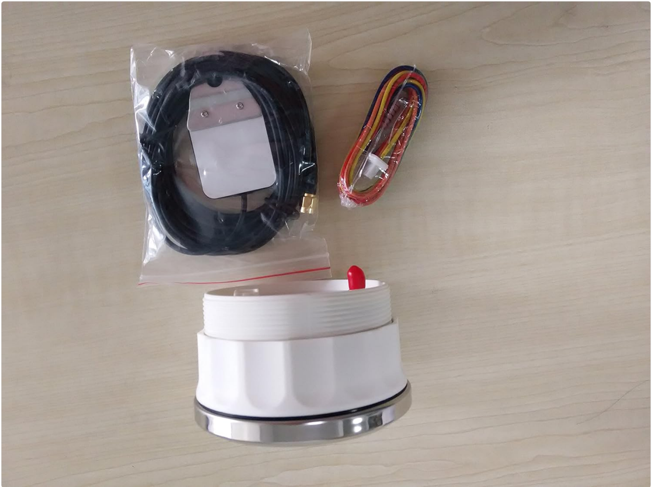
Figure 2: Contents of the KUS Digital GPS Speedometer Gauge package, showing the main gauge unit, the GPS antenna with its cable, and the electrical wiring harness.
