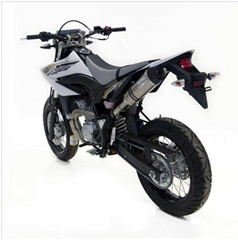
Figure 1: LEOVINCE SBK LV ONE EVO 2 Exhaust System. This image shows the complete exhaust system, including the silencer and link pipe, ready for installation on a motorcycle. Note the stainless steel finish and the distinctive design of the LV ONE EVO 2 series.
