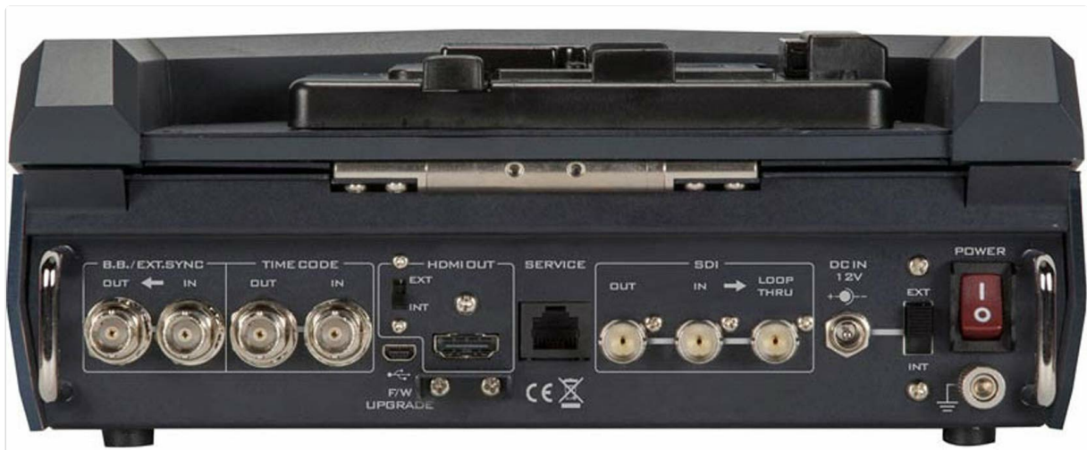
Figure 4.1: Rear panel connections of the Datavideo HRS-30, including SDI, HDMI, Timecode, and Power inputs/outputs.
