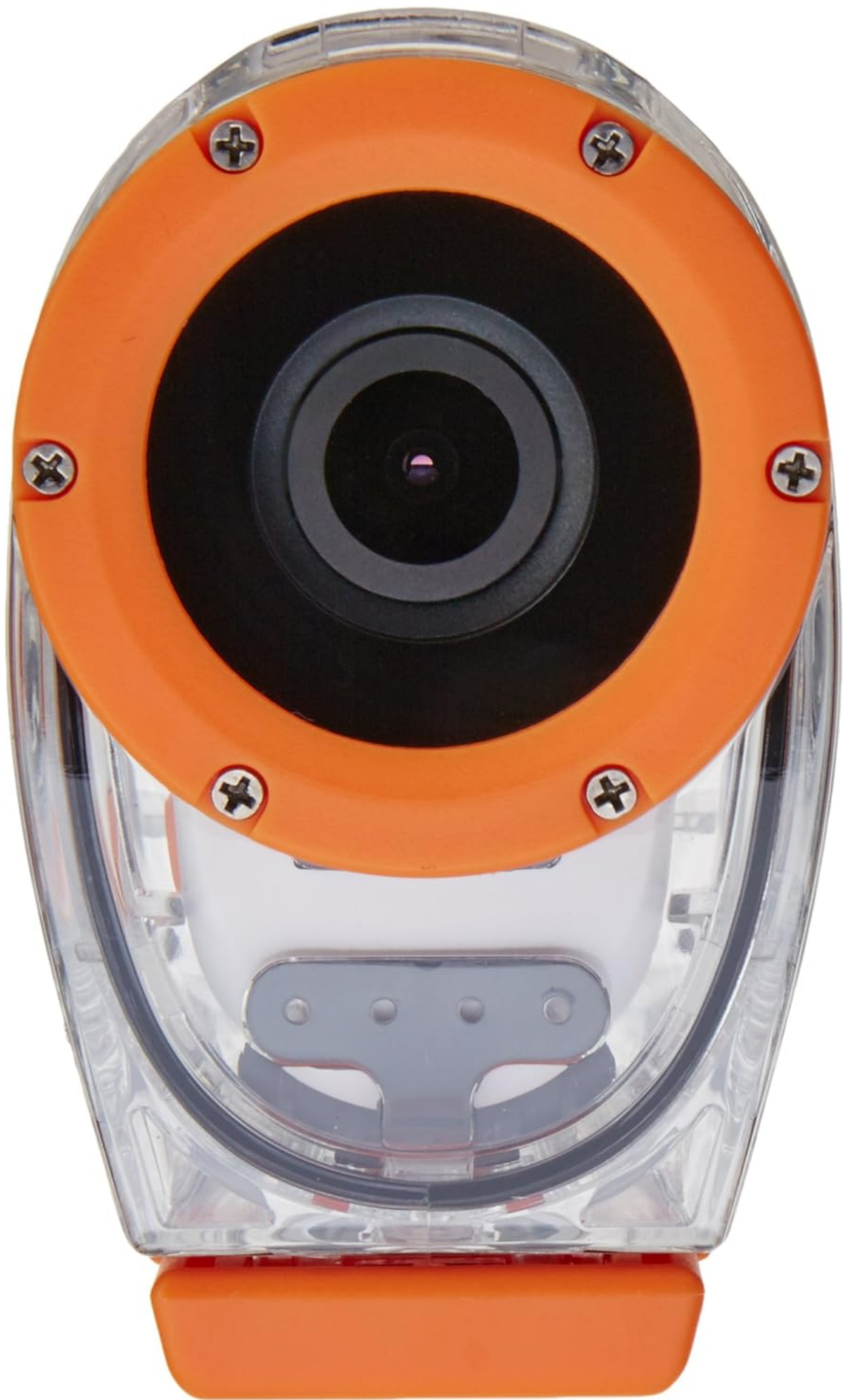
Figure 3: Front view of the camcorder, focusing on the fisheye lens and its protective orange ring.
