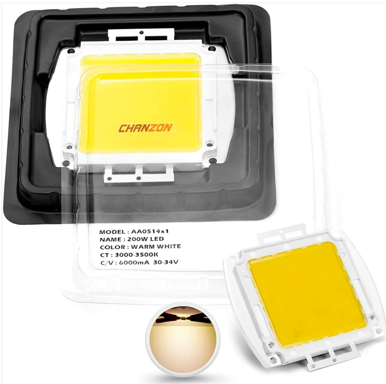
Image 7.1: CHANZON 200W LED Chip Packaging. This image shows the product in its clear plastic packaging, with a label indicating the model (AA0514x1), name (200W LED), color (Warm White 3000-3500K), and electrical specifications (6000mA, 30-34V).
