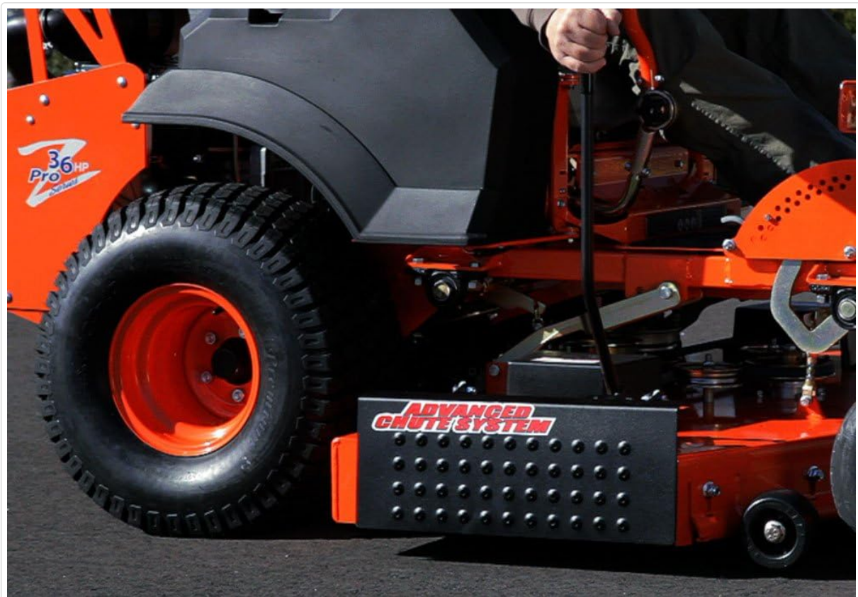
Figure 2: Advanced Chute System Chute Blocker installed on a zero-turn mower. This image shows the chute blocker mounted to the mower deck, ready for operation.
