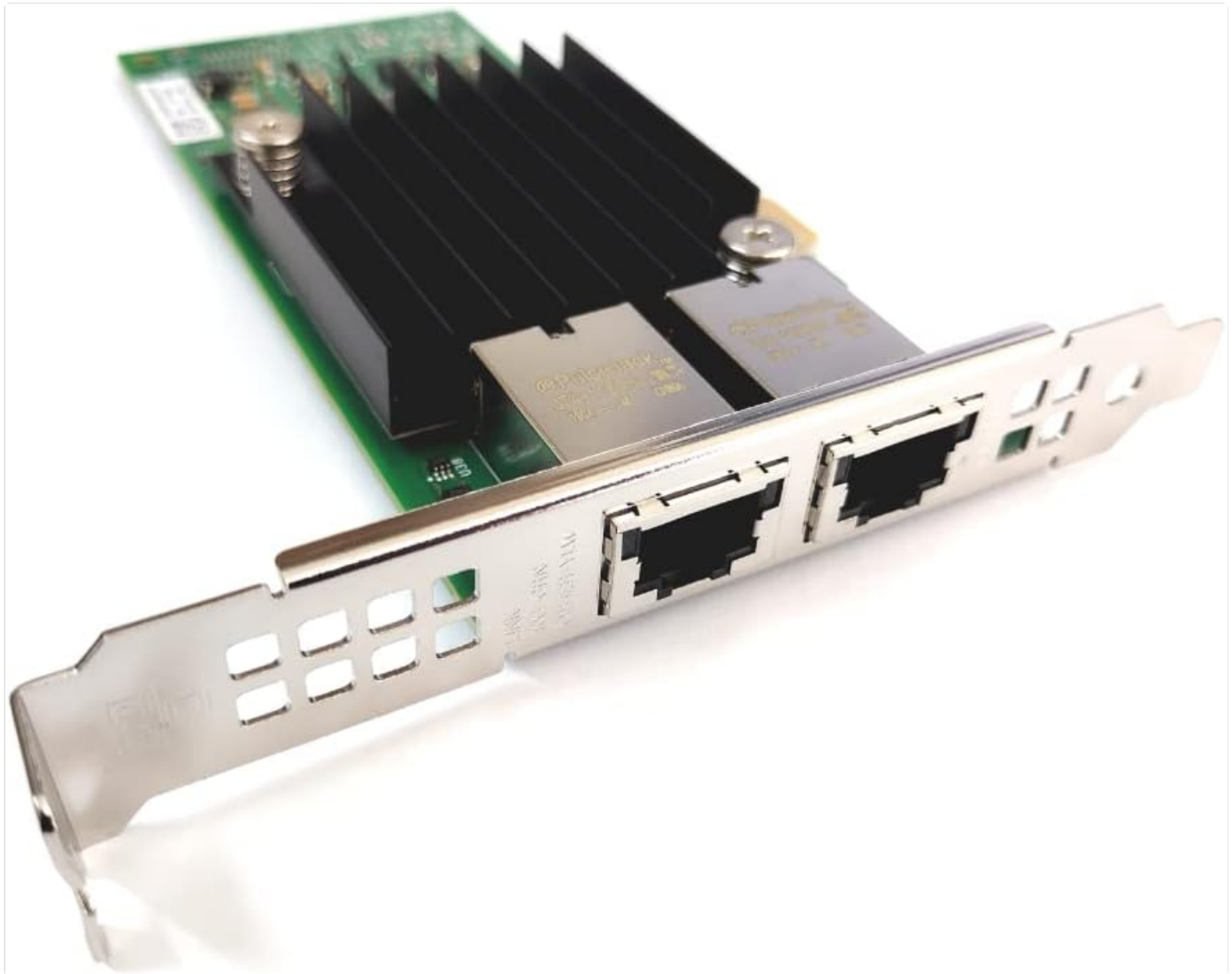
Figure 4.2: Close-up view of the dual RJ45 Ethernet ports on the Intel X550-T2 adapter, designed for 10GbE connectivity.
