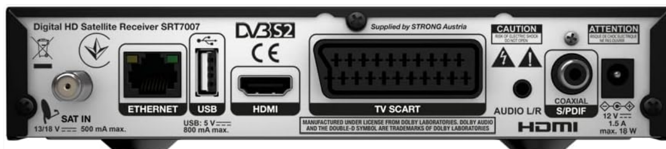
Figure 3.1: Rear panel of the receiver showing various input and output ports. From left to right: SAT IN, Ethernet, USB, HDMI, TV SCART, Audio L/R, Coaxial S/PDIF, and DC 12V power input.
