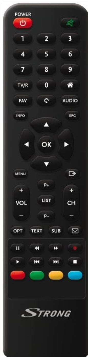
Figure 4.1: The remote control for the SRT 7007, featuring power, number keys, navigation, volume, channel, and media playback buttons.
