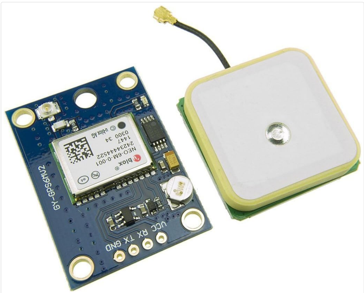
Figure 1: HiLetgo GY-NEO6MV2 GPS module with attached ceramic antenna.
