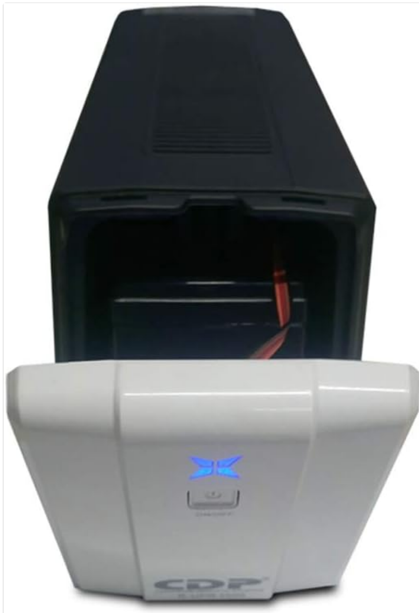
Figure 3: Top view of the UPS with the battery compartment open, showing the internal battery.
