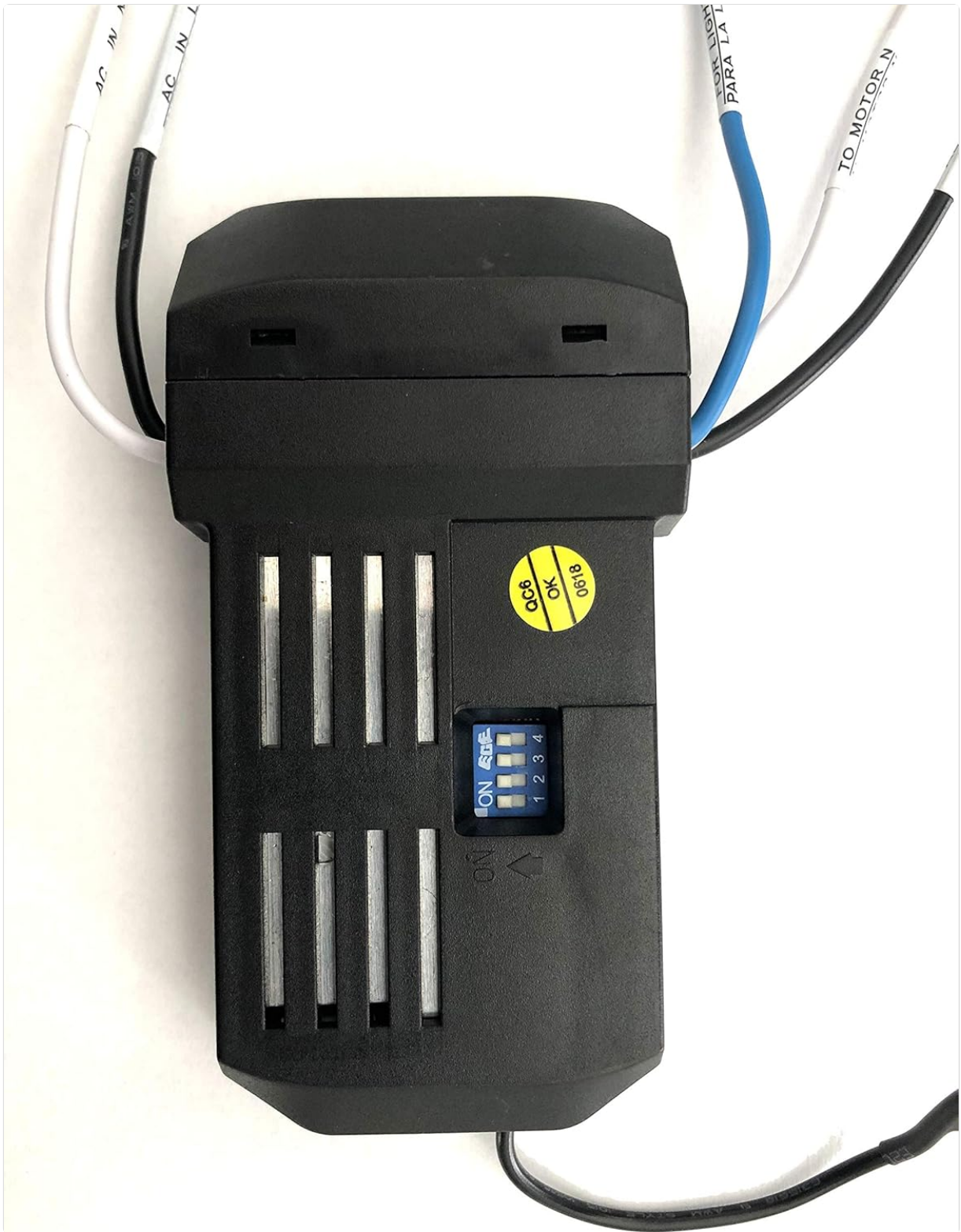
Figure 1: Front view of the Hampton Bay UC7067RC Remote Receiver, showing wiring connections and the DIP switch block for code setting.
