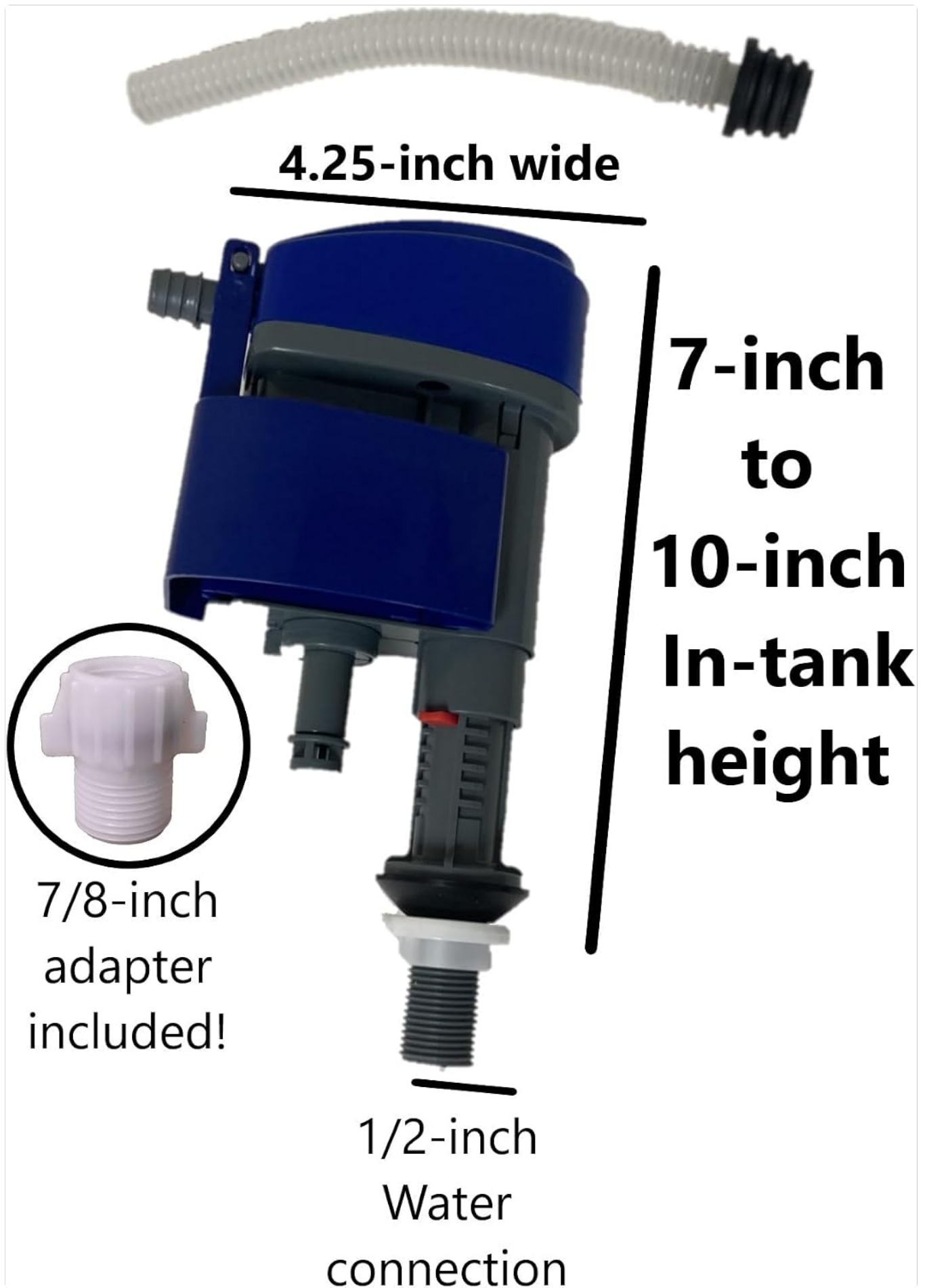
Figure 2.2: Front view of the NuFlush NFHDIVF Commercial Toilet Fill Valve, illustrating its adjustable height (7-10 inches in-tank) and width (4.25 inches), along with the 1/2-inch water connection and included 7/8-inch adapter.
